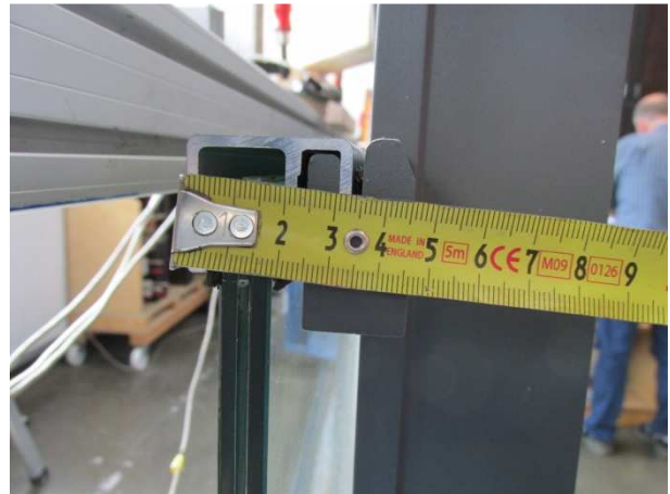
Picture 2 Cross section of the profile for glass holder
