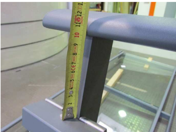
Picture 3 Distance of handrail to glass
