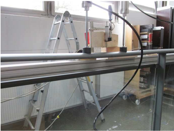
Picture 7 Static vertical test under load
